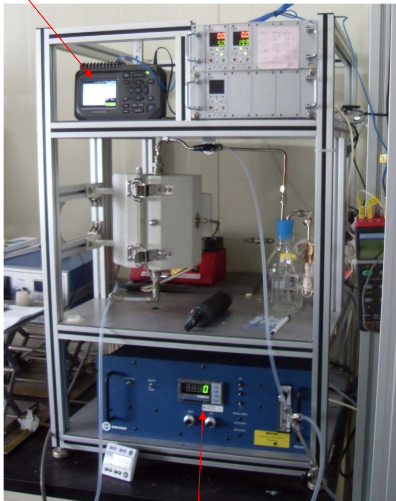
H 2 O 2 vapor analyzer (RM09-1000m, Interscan)
