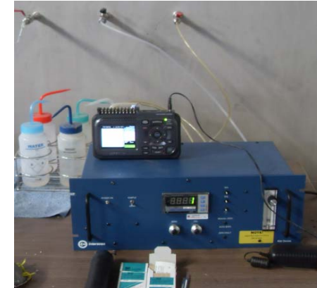
H 2 O 2 vapor analyzer (RM09-1000m, Interscan)
