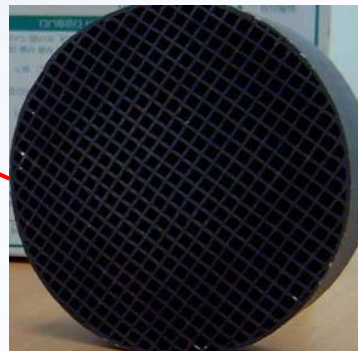
Catalyst installed into kerosene heater.
